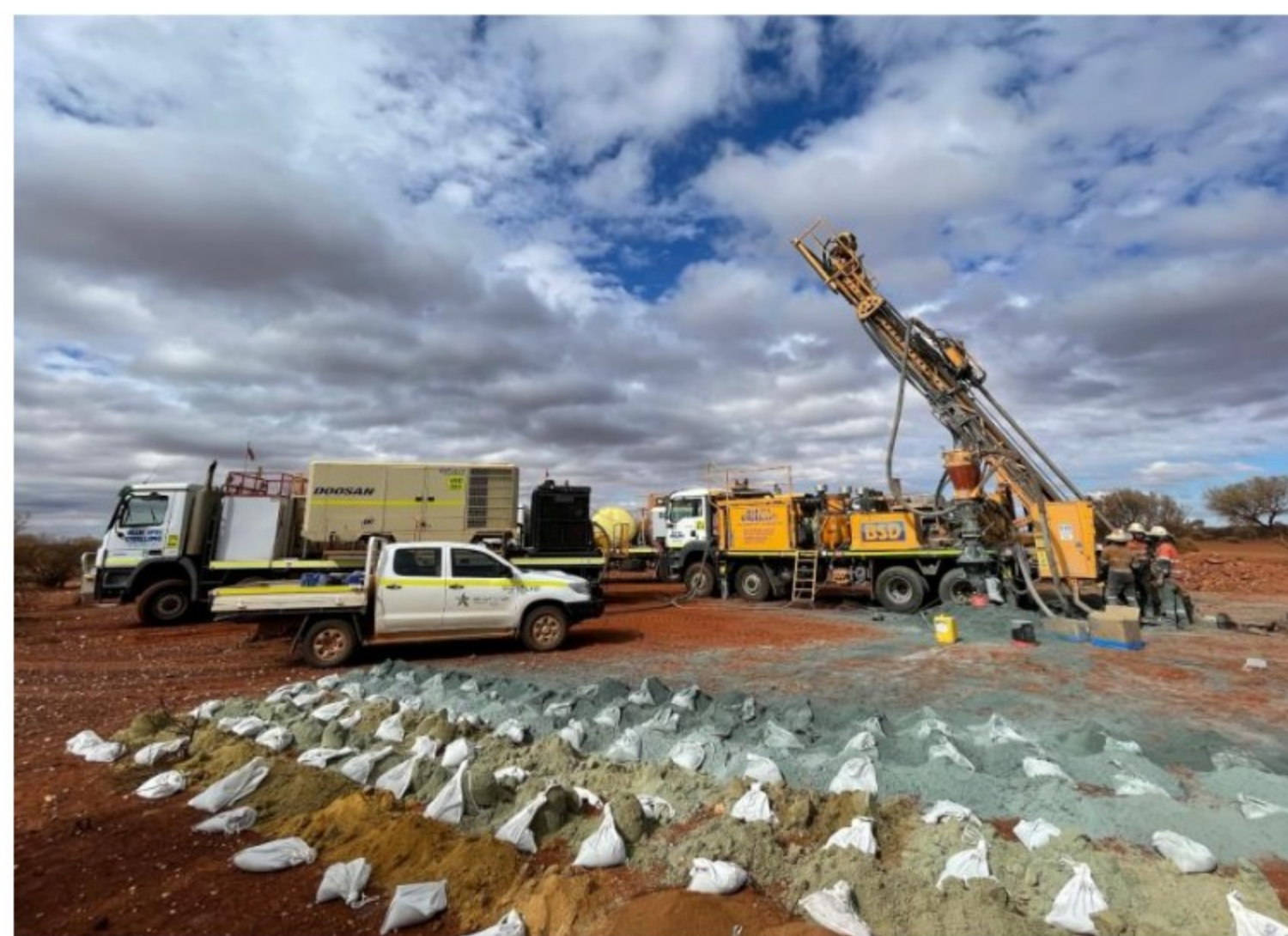
RC drilling operations at Brightstar Resources Cork Tree Well gold project in WA. Credit: File
