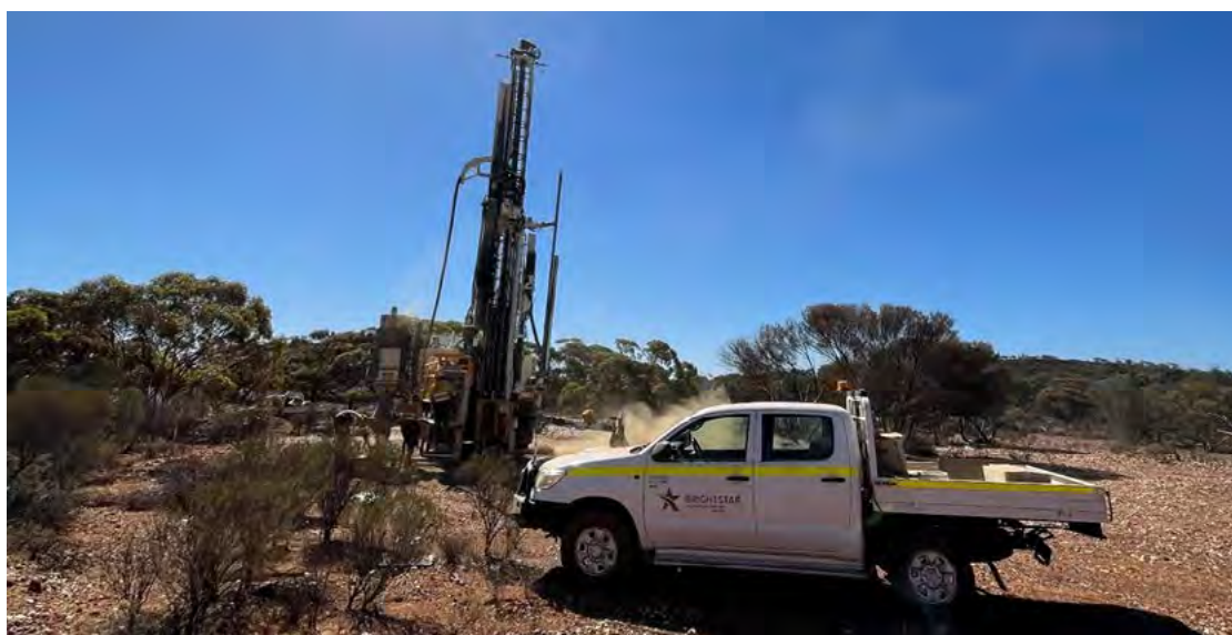
Figure 7: Aircore Drilling at Sailor Prince.
